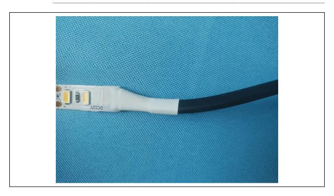
Details of: LED module of 12V-5730-120L-IP20
