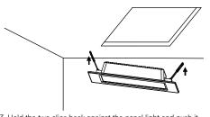
3. Hold the two clips back against the panel light and push it into the hole. Allow the springs to pull the light up to the ceiling.
