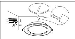
2.Switch OFF the power & Connect AC: 220-240V voltage with terminals.
