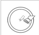
1. Power off, tap the central area of the diffusion plate with a pointed tool, and take out the cracked diffusion plate
