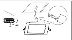
2.Switch OFF the power & Connect AC: 220-240V voltage with terminals.
