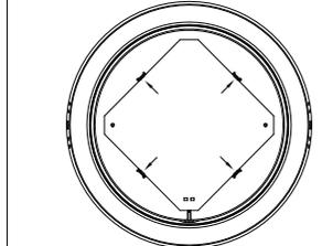
5. Press the buckle outwards, remove the aluminum substrate from the buckle, and remove the light source board.
