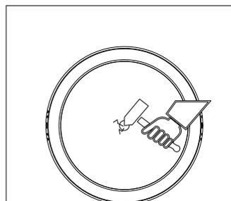
1. Power off, tap the central area of the diffusion plate with a pointed tool, and take out the cracked diffusion plate
