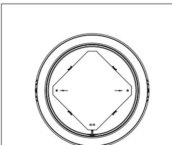
3. If there is no hot melt column in the lamp body or the hot melt column is not hot melt, this step will be adjusted without treatment. If the hot-melt column has been fused to fix the aluminum substrate, cut the hot-melt part of the hot-melt point with diagonal pliers.
