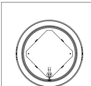
2. Remove the power wire from the plug terminal
