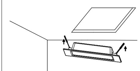
3. Hold the two clips back against the panel light and push it into the hole. Allow the springs to pull the light up to the ceiling.
