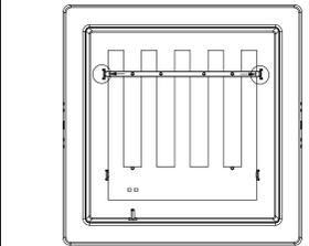
4. Press the buckle outwards, remove the aluminum substrate pressing strip from the bayonet, and remove the pressing strip. This step is only required for 24W panel light, other items are not required.
