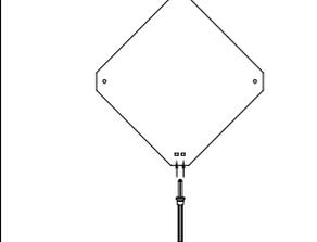
6. Take out two-cord cable (wire diameter 18-22AWG) and insert it into the plug-in terminal. Connect the external power supply for testing.
