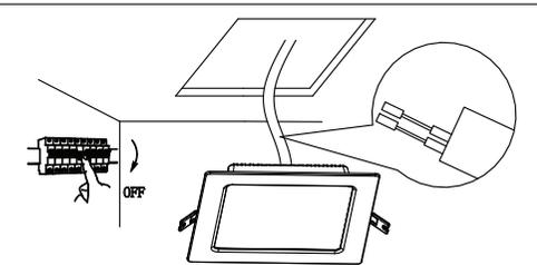
2. Switch OFF the power & Connect AC: 220-240V voltage with terminals.
