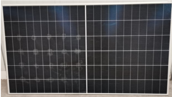
Sample 3-22#: Burning brand test (front)
