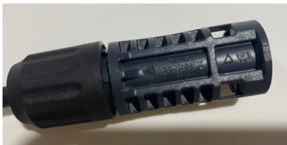
Mark (Do not disconnect under load)
