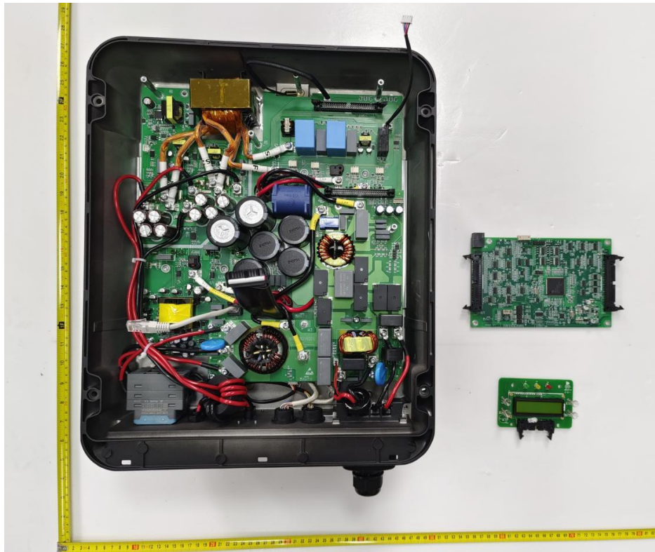
Internal view of inverter
