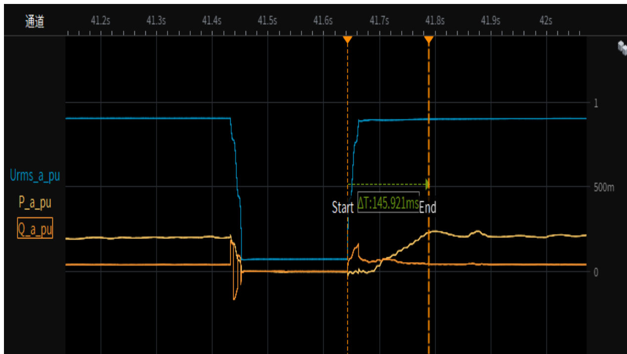
Test 1s-2.1 Depth of fault phase: 0.1p.u.,three-phase-symmetrical (type A),95% load Test overview(voltage,current,active and reactive power)
