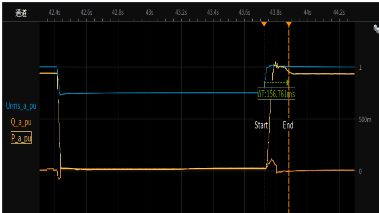
Test 4a-Depth of fault phase: 0.75p.u.,two-phase-asymmetrical (type D), 0% load Test overview(voltage,current,active and reactive power)
