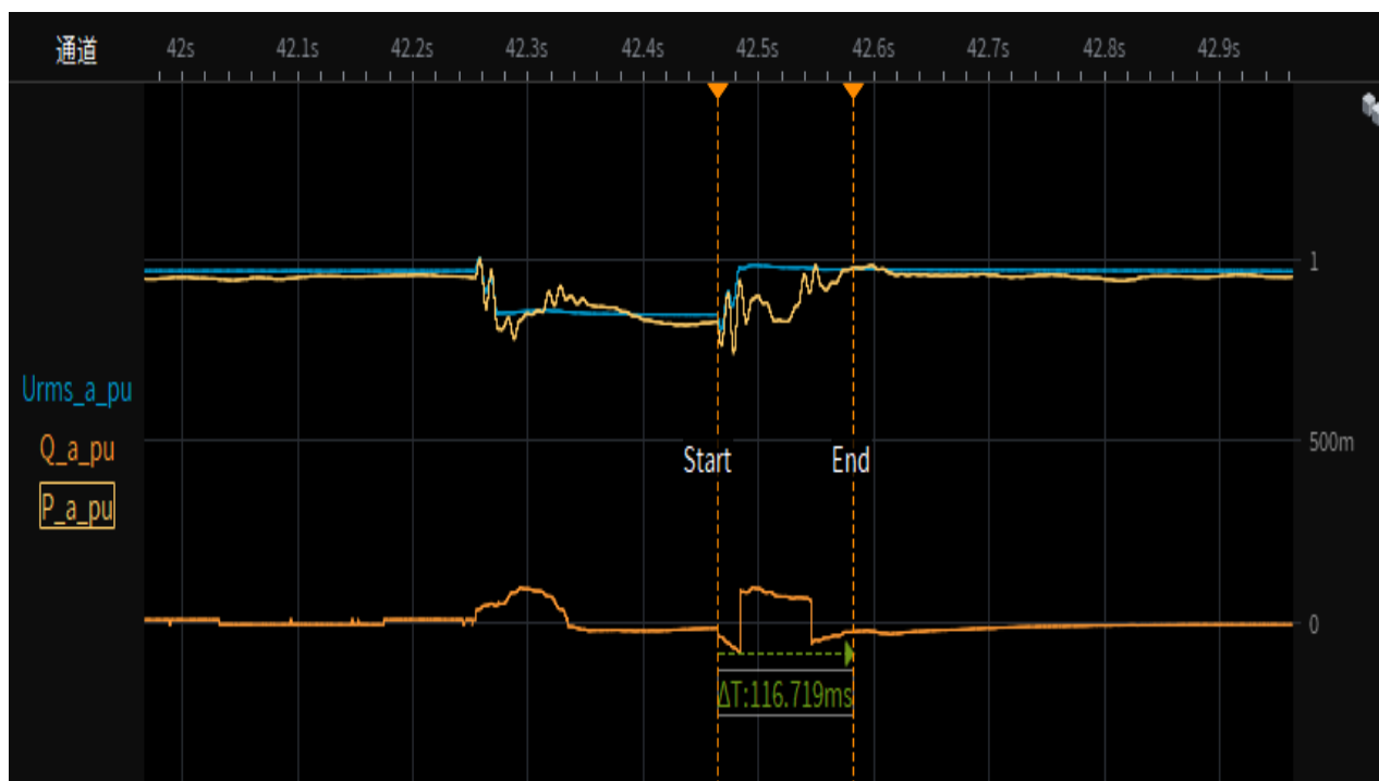
Test 1a-2.4 Depth of fault phase: 0.1p.u., two-phase-asymmetrical (type D), 95% load restoring time
