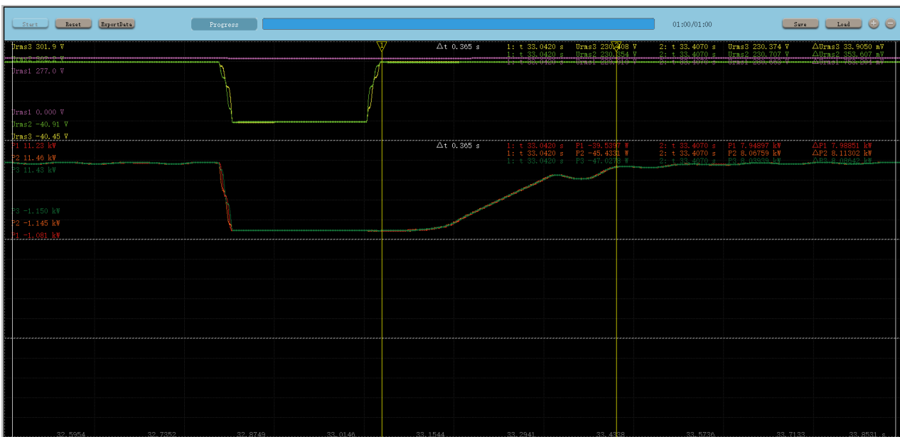
Test number 6, 50%Vn, 850ms, asymmetrical two-phase LV fault
