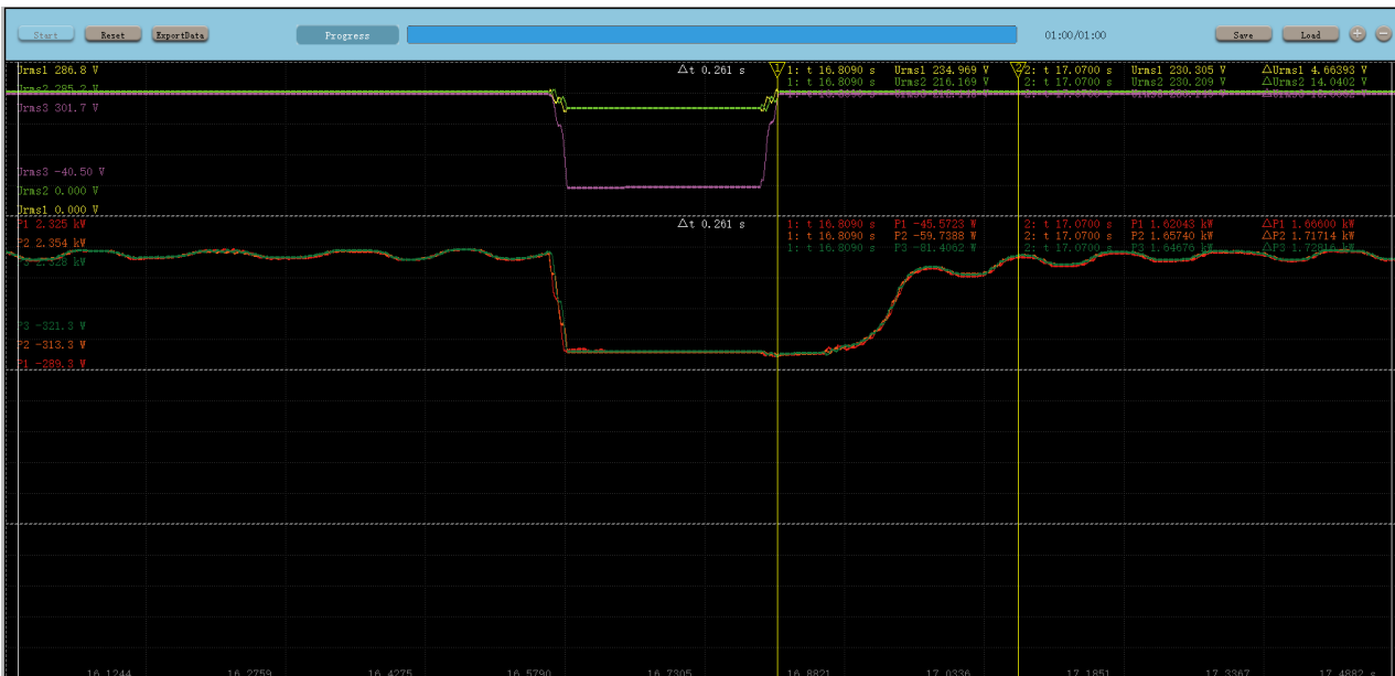
Test number 2a, 25%Vn, 400ms, asymmetrical two-phase fault
