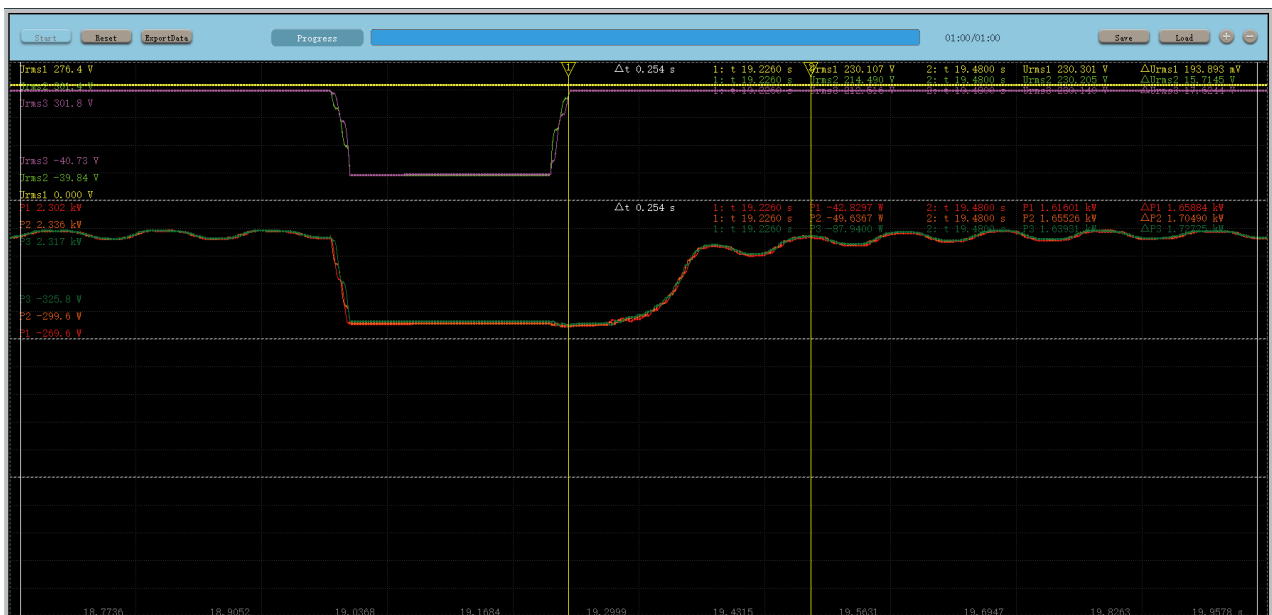
Test number 6, 50%Vn, 850ms, asymmetrical two-phase LV fault
