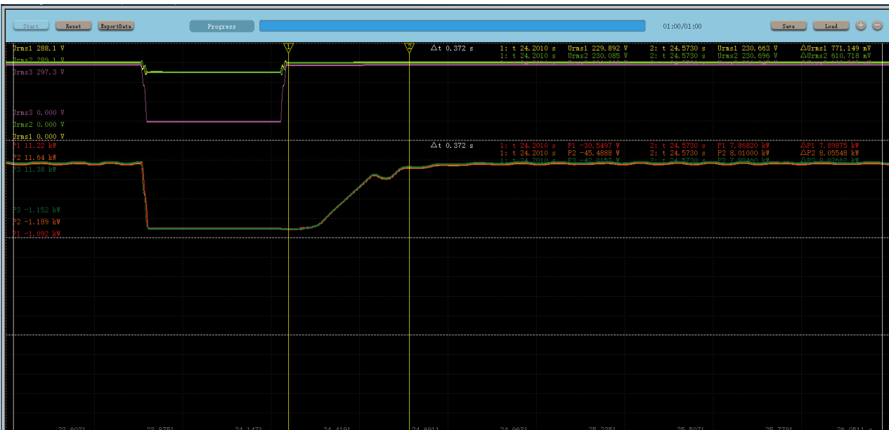
Test number 3a, 50%Vn, 850ms, asymmetrical two-phase fault
