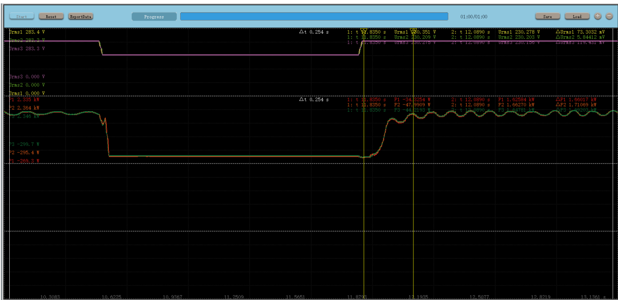
Test number 1a, 10%Vn, 200ms, asymmetrical two-phase fault
