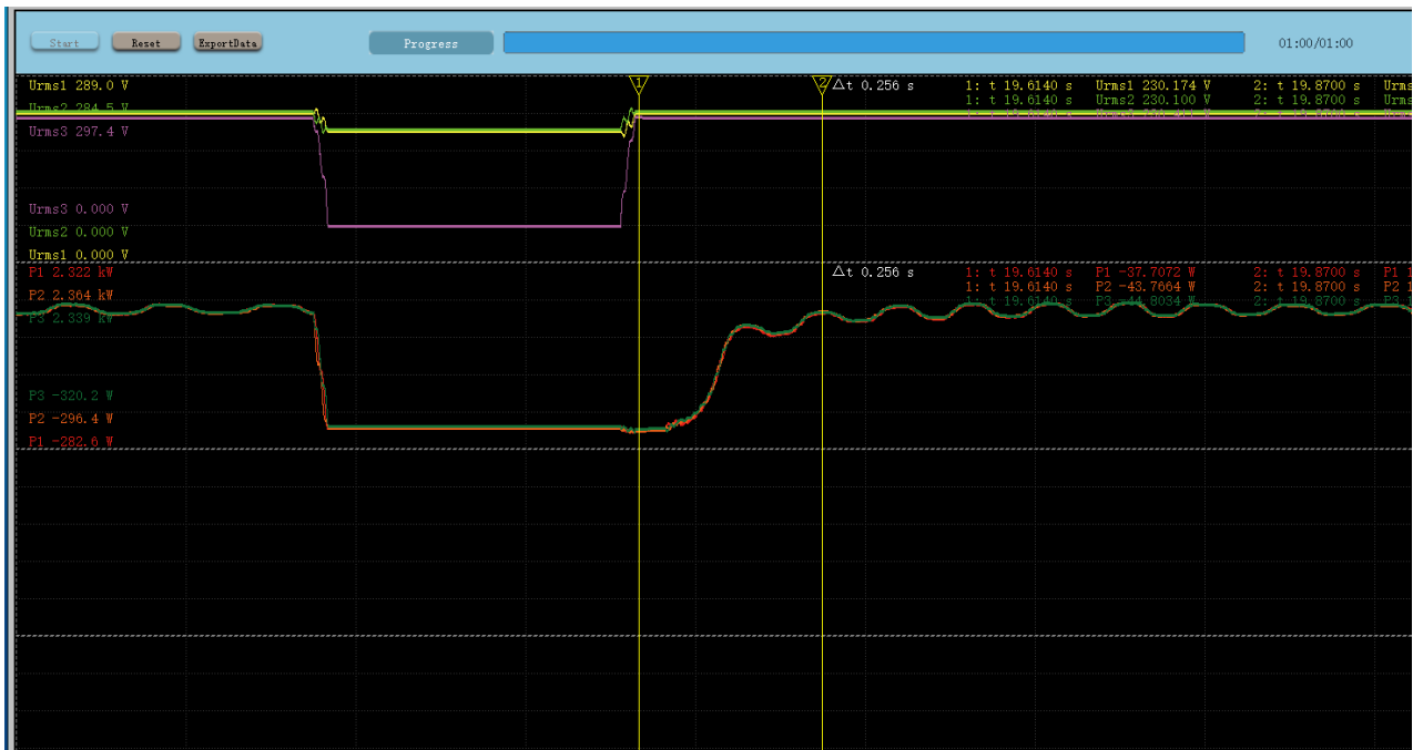
Test number 3a, 50%Vn, 850ms, asymmetrical ltwo-phase fault
