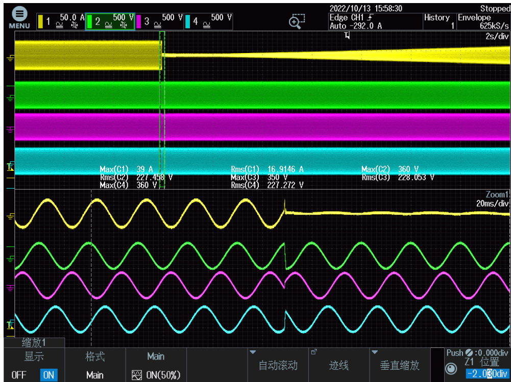
Current curve at 180° phase shift (@100% Pn):
