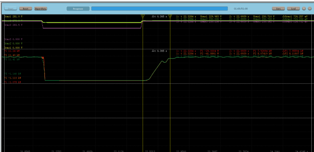
Test number 5, 10%Vn, 200ms, asymmetrical two-phase LV fault
