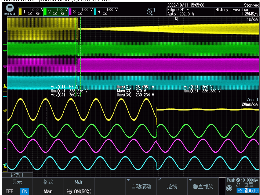
Current curve at 180° phase shift @33% Pn):
