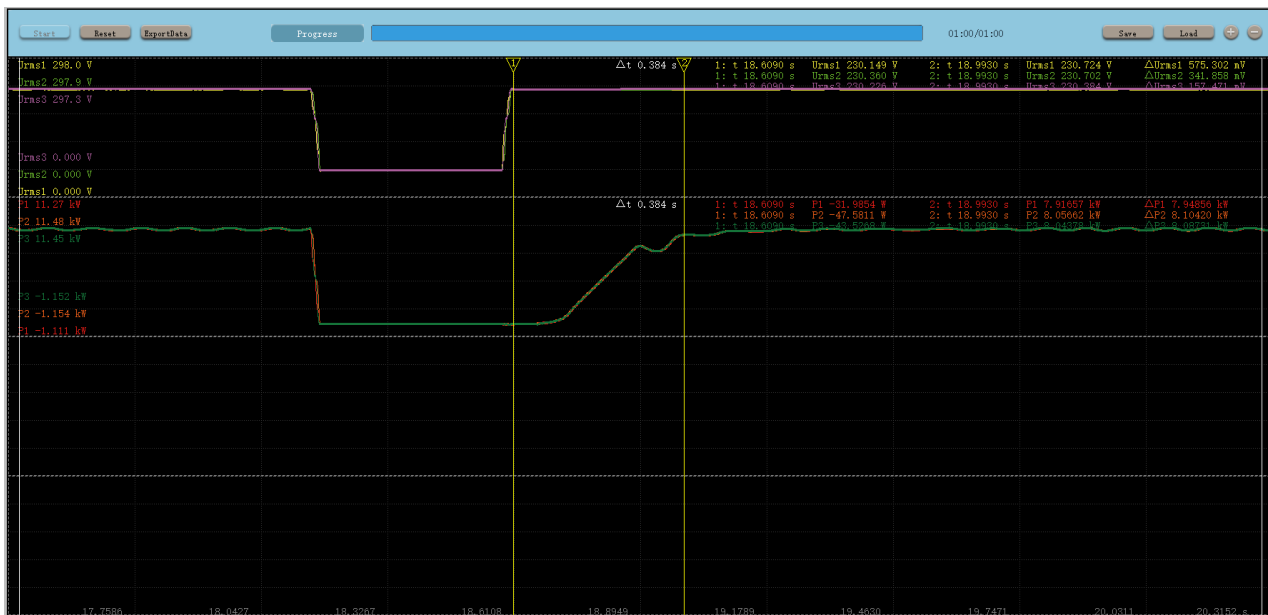
Test number 3s, 50%Vn, 850ms, three-phase symmetrical fault
