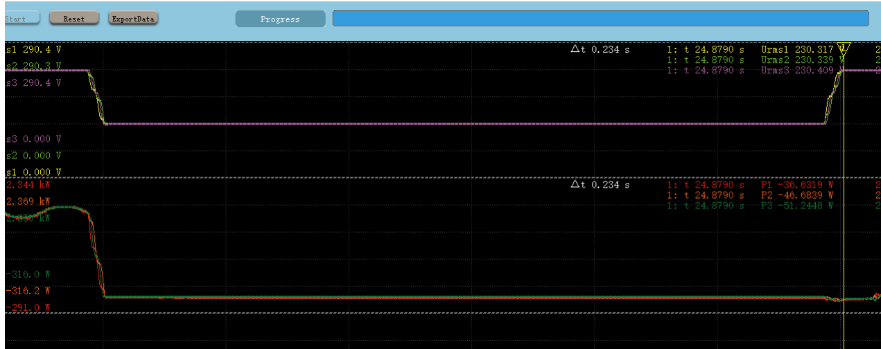
Test number 4s, 75%Vn, 1300ms, three-phase symmetrical fault
