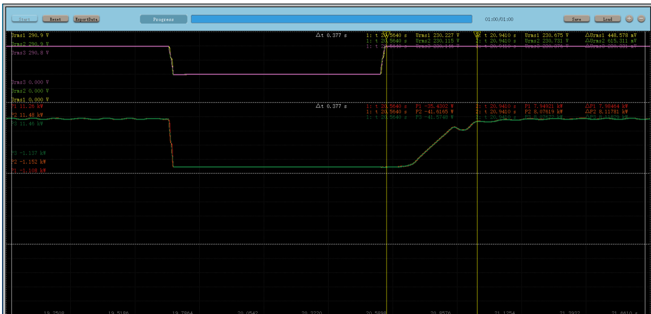
Test number 4s, 75%Vn, 1300ms, three-phase symmetrical fault
