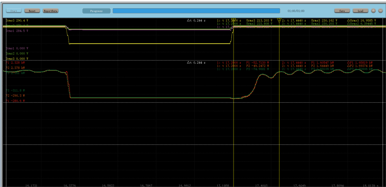
Test number 4a, 75%Vn, 1300ms, asymmetrical two-phase fault
