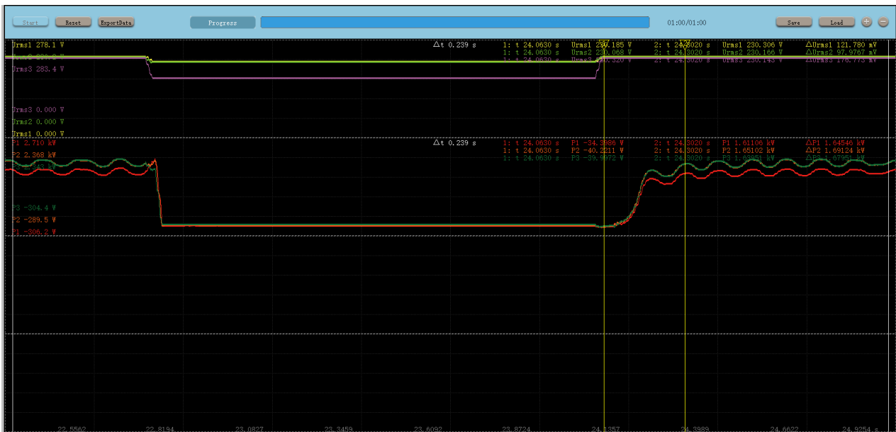
Test number 5, 10% V_n , 200ms, asymmetrical two-phase LV fault
