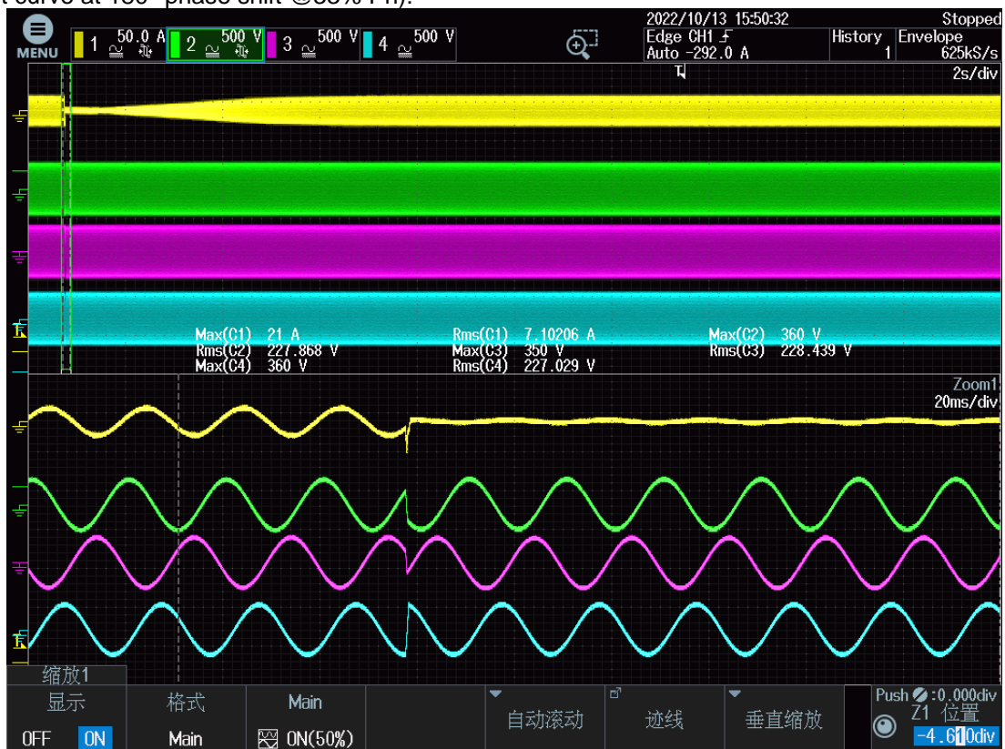
Current curve at 180° phase shift @33% Pn):
