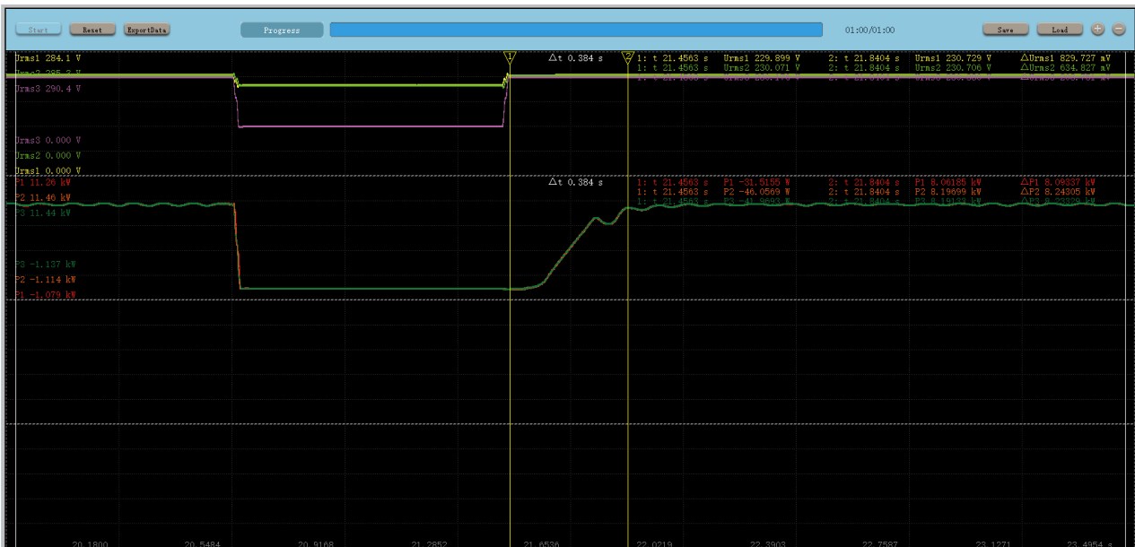
Test number 4a, 75%Vn, 1300ms, asymmetrical two-phase fault
