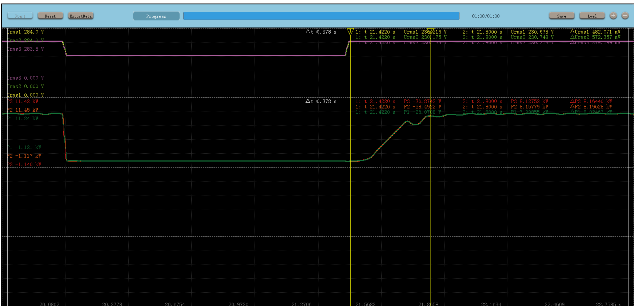
Test number 1a, 10%Vn, 200ms, asymmetrical two-phase fault
