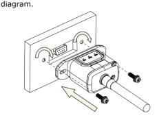
Type 2 Step1: Assemble logger to the inverter communication interface as shown in the diagram.
