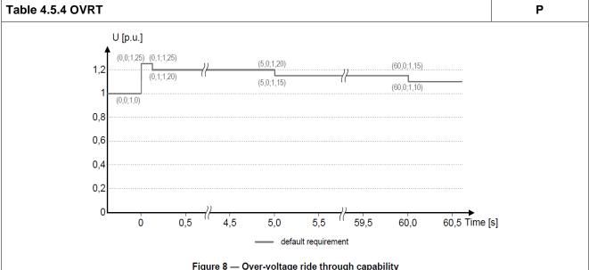
Figure 8 — Over-voltage ride through capability
