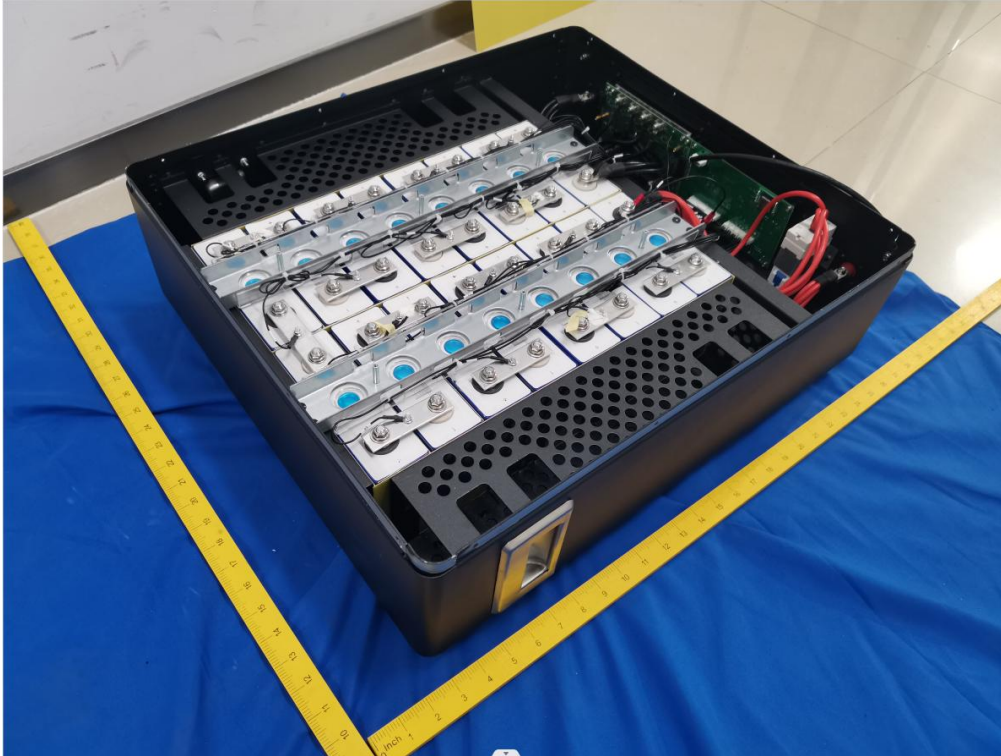
Figure 5 Inside view of battery
