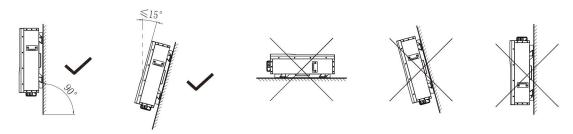
In order to ensure good heat dissipation of the machine and convenient operation and maintenance of personnel, sufficient clearance shall be reserved for the machine during installation. The specific requirements are shown in the figure below:
