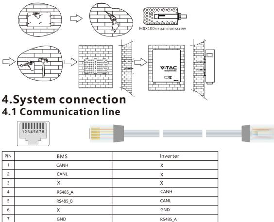
• Different inverter communication protocols have different pin definitions. Please pay attention to the compatibility between the battery and inverter RS485 / can communication line.
