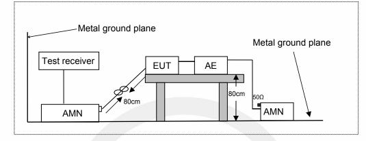
AMN: Artificial Mains Network AE: Associated equipment EUT: Equipment under test
