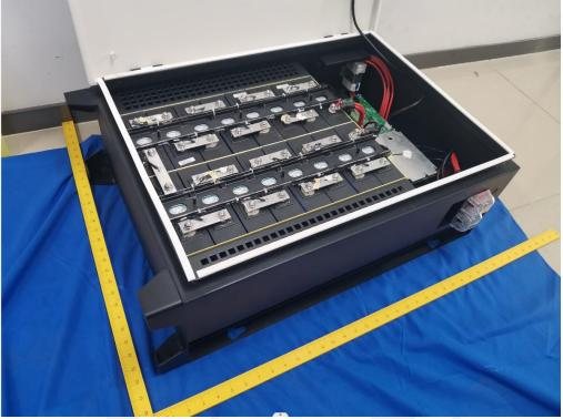
Figure 5 Inside view of battery
